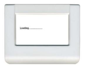
This screen indicates that the firmware is now being loaded. This takes approximately 1 - 2 minutes. The USB drive should be removed at this point.
